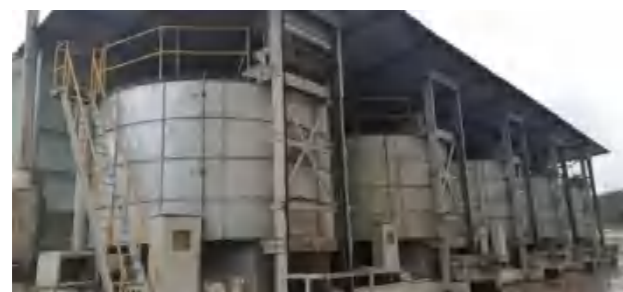
Figure 5-1-3-7 Smart composting tank for organic fertiliser
